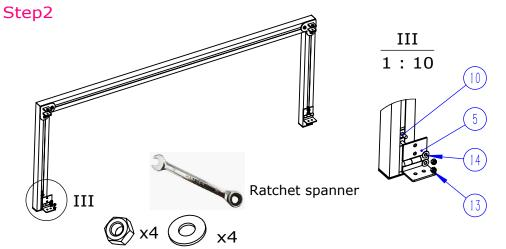
Insert the Latches of the SS Hinge (5) to the holes on the Front Frame (1). Use the Slide Blocks (10), M8 Lock Nuts (13) and Washers (14) to fix the SS Hinge to the Front Frame. Note: Do not over tighten the bolt.
