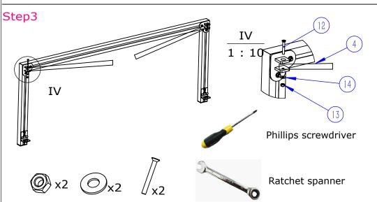
Insert the PP Bows (4) into the Alu PLate of the Heart Casting (3). Use the M8 x 60 Countersunk Bolts (12), Washers (14) and Lock Nuts (13)to fix the PP Bows (4) to the Front Frame.
