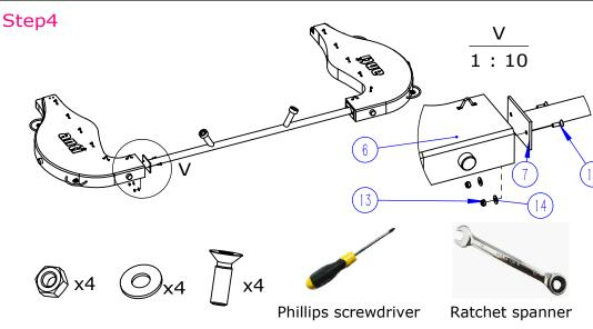
Use the M8 x 30 Countersunk Bolt (11), Washers (14) and Lock Nuts (13) to fix the Small GRP Floats (6) to the Back Tube (7).
