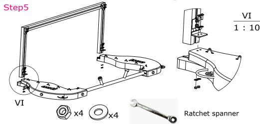
Slide the Slide Blocks (10) as shown above into the top corner of the front frame. Slip the Alu Heart Casting (3) into the slide blocks and connect using the M8 Waster (14) and Lock Nut (13) to fix to the frame.
