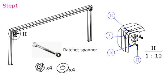
Slide the Slide Blocks (10) as shown above into the top corner of the front frame. Slip the Álu Heart Casting (3) into the slide blocks and connect using the M8 Waster (14) and Lock Nut (13) to fix to the frame.
