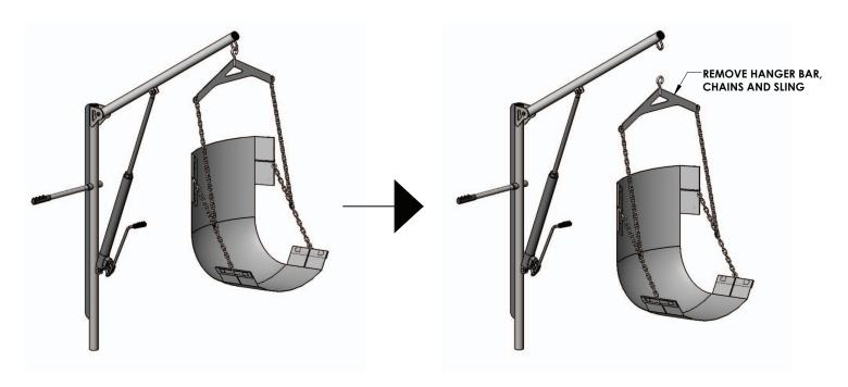
Once the sling seat has been removed, add the quick link to the u-bolt that is attached to the lifts boom arm. Then, attach the 4-point hanger bar to the quick link followed by connecting the chains and hard seat to the 4-point hanger bar. All pools and spas are different so the chains may have to be adjusted slightly to fit specific applications and/or personal needs.
