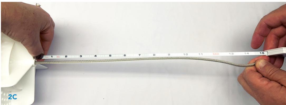
*\*The EZ-Tensioner is 2.5" longer than the current take-up reel. A few discs and/or donuts may need to be removed to accommodate the NEW EZ-Tensioner.*
