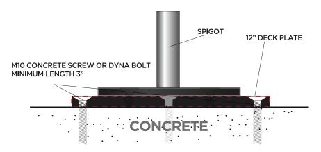
**IMPORTANT:** CONCRETE SLAB SHOULD HAVE A MINIMUM DEPTH OF 6".
