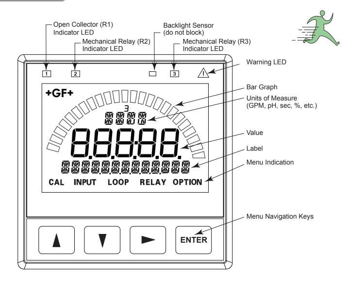
All possible segments shown in this illustration. The instrument's software controls which segments are shown at any particular time. Only the bar graph and GF logo are visible when the unit is turned off.
