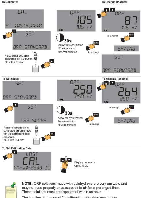
The solution can be used for calibrating more than one sensor. However, the solution must remain free of debris and must not be diluted by rinse water from previous calibrations.
