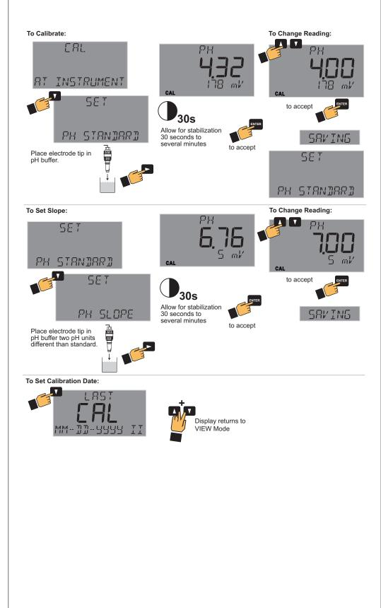
Single-point calibration sets STANDARD only; Signet recommends a two-point calibration to set SLOPE in addition to STANDARD.
