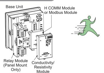
If the 9900 Base Unit will be mounted in a panel, the plug-in modules may be installed either before or after the base unit is mounted. If the 9900 Base Unit will be mounted using the wall mount accessory kit (3-9900.392), install plug-in modules first.
