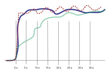
Averaging is different depending on the measurement type. Seconds to 95% of Final Value for Low, Med, and High are:
