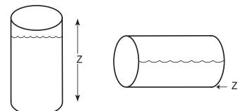
For most vessels, the zero reference point (Z) may be designated as any height in the vessel.
