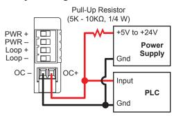
If PLC needs 0 logic input when relay is not energized, set NORMAL to CLOSED in the RELAY menu when using the Open Collector (R1) with NPN style wiring.
