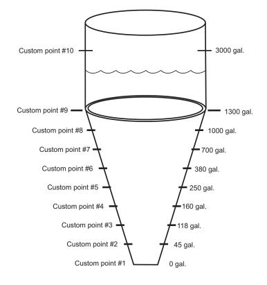
In the LEVEL/VOLUME INPUT menu (see page 41), if SHAPE is set to HORIZ CYLINDER, RECTANGLE or CUSTOM, the tank shape can be defined with the following screens:
